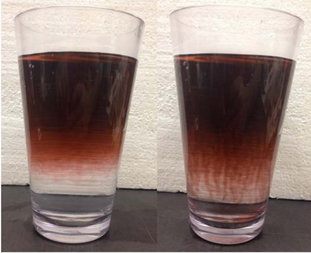
Figure 3. Salt fingers. As a sample miniature experiment, a cup was initially filled with warm salty colored water on top and cold fresh clear water below (left). After several minutes, salt fingers had formed and colored fingers could be seen growing downwards (right).
